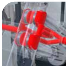
Power backflush filter with adjustable operation of melt accumulators
