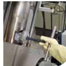
Entire surface of the piston can be cleaned – this ensures easy maintenance and long service life
