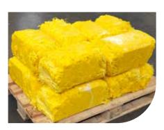
The end product of the Starlinger compSTAR are compacted blocks of endless tapes with 90 % volume reduction, minimised risk of contamination and easier handling of the otherwise loose endless tapes.
